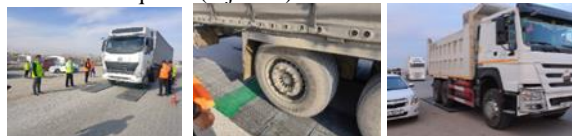
3– rasm. M-39 "Almata-Bishkek-Toshkent-Shahrisabz-Termiz" avtomobil yo'lining 1402 km da og'ir yuk transport vositalarining vaznini TENZO mobil tarozida o'lchov ishlari
