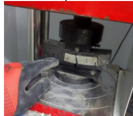
Figure 3. Bending test of specimens
