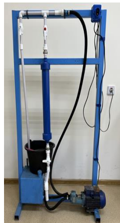
1-elektr dvigateli, 2-moy nasosi, 3-sinalayotgan filtr, 4-filtrlangan moy idishi, 5-moy idishi 4-rasm. Moy filtrlarini sinovdan o'tkazishning sxemaga asoslangan stendi (a) va uning sxematik ko'rinishi ta'svirlangan (b)
