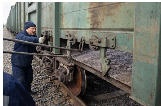
1-rasm. Yarim ochiq vagonning quyi lyuklari yuk tushirish jarayonidan lavhalar
