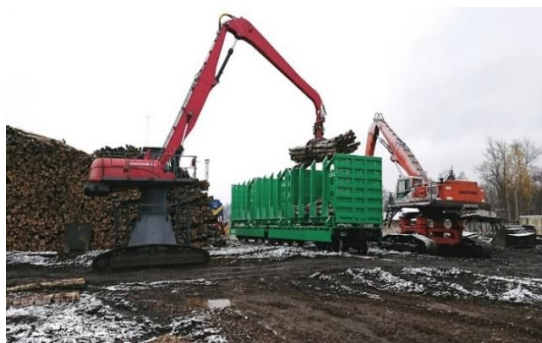
1-rasm. Yog'och materiallarni tashish uchun mo'ljallangan almashinuvchi kuzov
