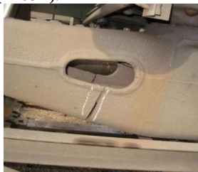
4-rasm. Ressor osti balkasida charchash natijasida yuzaga keladigan yoriq
