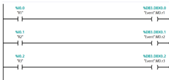
9-rasm LD (Ladder Diagram) tilida yozilgan dastur namunasi
