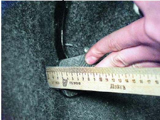
1-rasm. b) Tormoz tepkisini oxirigacha bosishdagi o'lchami
