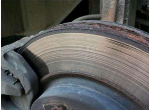
3-rasm. c) Noto'g'ri yeyilishdagi shovqin
