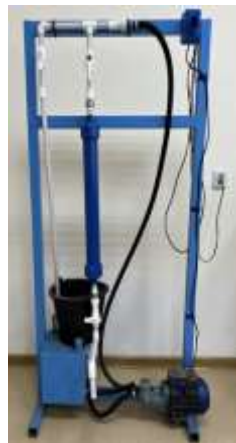
1-elektr dvigateli, 2-moy nasosi, 3-sinalayotgan filtr, 4-filtrlangan moy idishi, 5-moy idishi 4-rasm. Moy filtrlarini sinovdan o'tkazishning sxemaga asoslangan stendi (a) va uning sxematik ko'rinishi ta'svirlangan (b)
