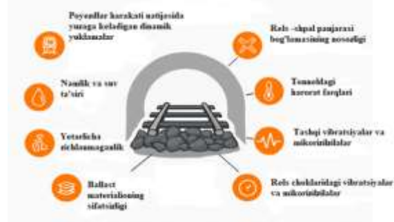
2-rasm. Ballast prizmasining nosozligini keltirib chiqaruvchi omillar
