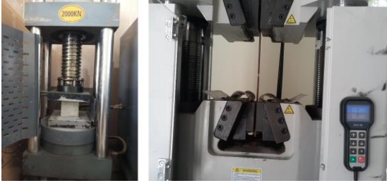
3-rasm. Beton kublarni (a) va armaturani (b) sinash
