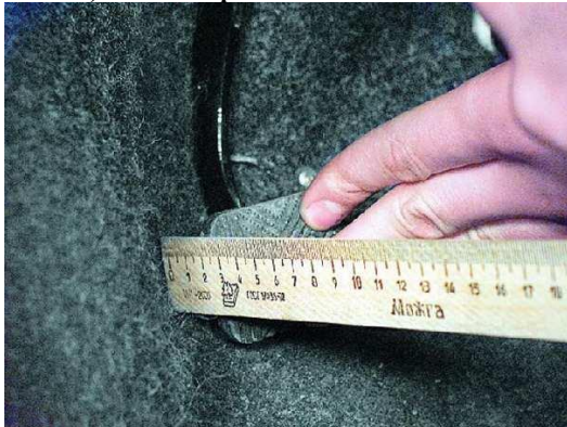
1-rasm. b) Tormoz tepkisini oxirigacha bosishdagi o'lchami
