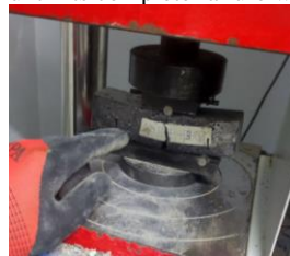
Figure 3. Bending test of specimens
