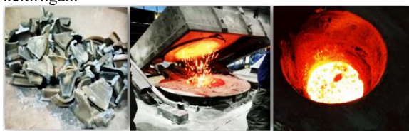
1-rasm. Induksion tigel pechida ikkilamchi xom ashyolardan foydalanib sintetik cho'yan eritish jarayoni
