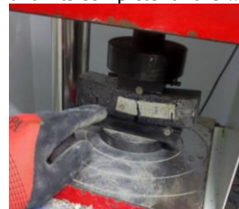
Figure 3. Bending test of specimens
